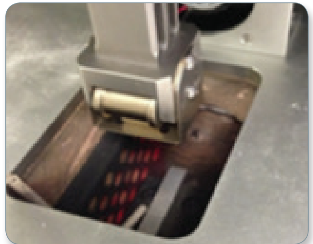
Figure 1. Passive roller system used for simulation of hot rolling.
